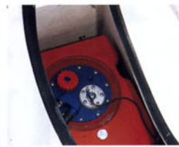
Twin fuel tanks are in the seat bases.
